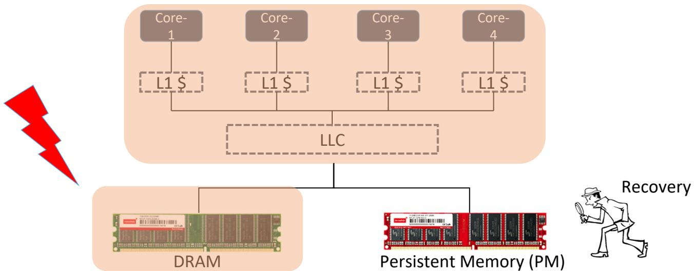
**Recovery can inspect the data-structures in PM to restore system to a consistent state**
