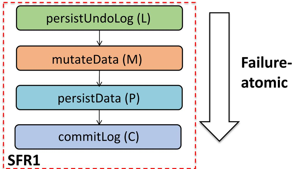
**Need to ensure the ordering of steps in undo-logging for SFRs to be failure-atomic**
